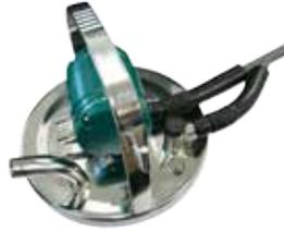
5. Connect long blue stripe hose from the stallcock (1/4 turn valve) on the vacuum pump handle to the grey plastic hose port "Y" at the bucket lid. The lid comes with pulsator and milking unit prebuilt.
